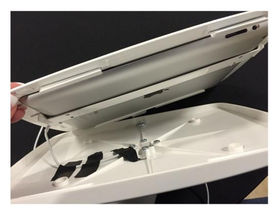
The iPad "frame" has two metal "clips" (see page 3) that slide into place with the base. This part is somewhat tricky ... so take it slow, making sure that the clips slide into place, and the power cord is not caught in the edge of the frame. The iPad frame will "snap" into place when everything is lined up correctly.
