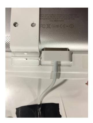
To plug the iPad in, slide the connector into the power slot on the bottom of the tablet. This isn't hard to do, but it can be awkward the first few times you try. Please do \*not\* untape the cord from the case. The connector will only work one way, so if it doesn't slide in easily, turn it over and try again.
